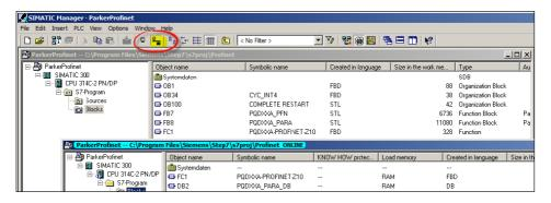
Copy the instance DB of the PARA block by drag & drop from the online to the offline folder. A message will pop up which can be acknowledged (Yes).
