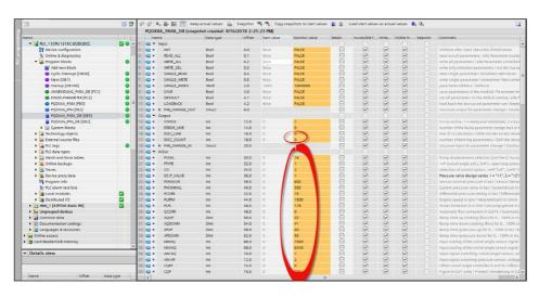
Next step is the setting of parameter PVSEL, (P)TYPE, CO and DS:P\_VALVE which are driving underneath laying parameter and functions. The "WRITE SEL" command writes the mentioned
