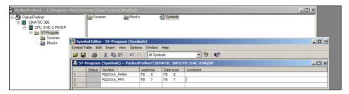
Translate the source by right – click and "Compile" before using the function block in the PLC user program (function):
