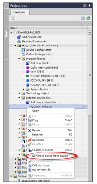
Generate the function block from just imported external file with the right mouse button dialog. The function block is ready to use in the "Program blocks" folder after compilation. The function blocks number may differ. The parameter
