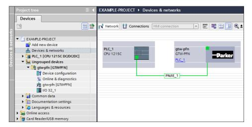
Check if the 32 byte I/O has been installed correctly under device and network (Device view).
