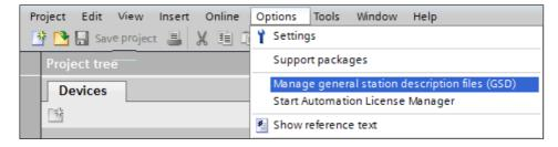
Point to source path of the just downloaded GSDML file, select the file in the content list and press install.
