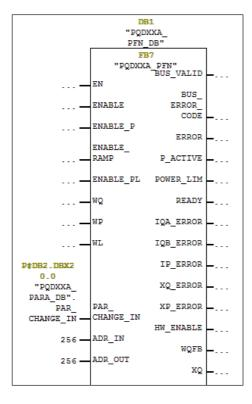
As well as the structure variable PQDXXA\_PFN\_DB.PAR\_CHANGE\_OUT to the input "PAR\_CHANGE\_OUT" of the parametrization FB:
