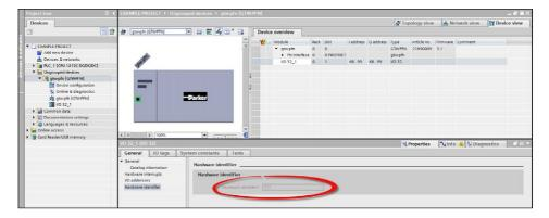
The driver function block is delivered in SCL format (File: PQDXXA\_PFN.scl) and need to be installed in TIA Portal as external source file.
