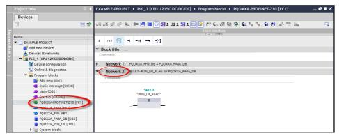
Due to the internal handling of the instance data block as image of the set values it is not recommended to use the data block in form of a multi instance.
