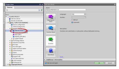
While installing the function block by drag and drop in the just created function / network a new instance data block gets created where the function block saves its data to.
