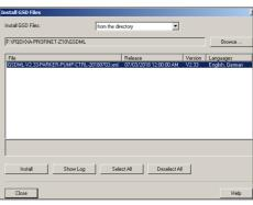
The PQDXXA-Z10-PROFINET appears in the hardware catalogue accordingly for implementation in the network under: PROFINET IO\Additional Field Devices\ Controllers\PUMP-CONTROLLER\GTW-PFN.
